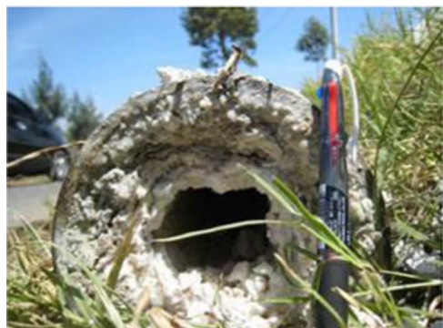
Fig. 5. Silica scaling in Dieng power plant, which is an obstacle of fluid flow [35].
